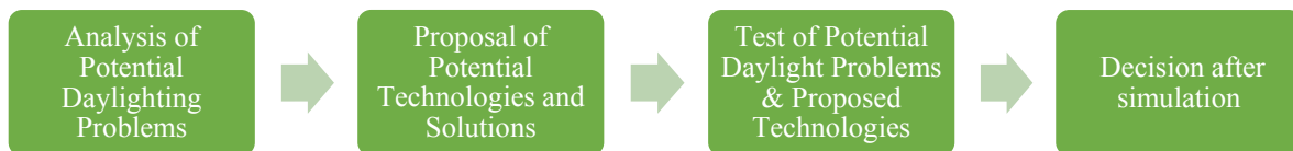
Figure 1. Workflow for the daylight design approach that is projected to form a methodology for IPD (Integrated Project Delivery) practice.
