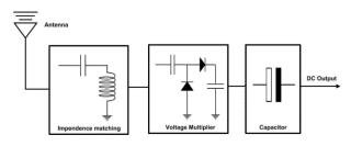
Fig. 1. General architecture of RF energy harvesting system.
