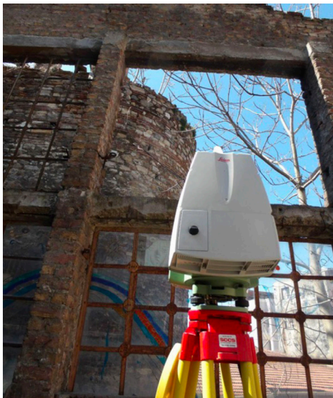
Fig. 6- The scanner unit at work from the buildings around tower two
