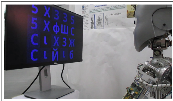
Figure 10. Experimental setup: the iCub robot and a scene for visual perception.
